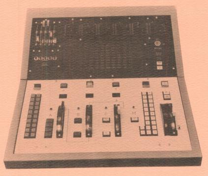
• Channel Level Indicator. When any channel number is selected, its working level is shown by the illumination of a number of LED indicators mounted alongside the channel fader scale. These form a luminous column the height of which corresponds to the level for that channel.
