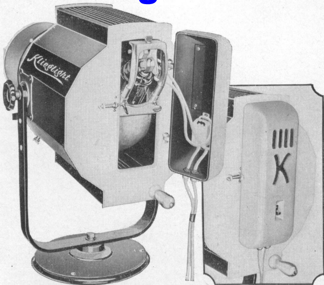
Rear view of new Klieglight, showing removable lamp holder, especially devised to firmly hold the bipost base lamp in a fixed prefocused position—adjustments being provided for properly locating the lamp to procure an even distribution of light. Insert shows the 25-ampere snap switch as mounted in the hinged back casing of the Klieglight, and the control handle for directing the light beam.
